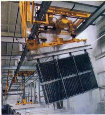
▲ Parts on titanium racks are moved down the line on one of six 4000 lb. capacity automatic hoists.
