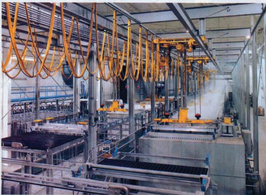
▲ Walgren's 290 ft. anodizing line, installed at Pioneer Metal Finishing's Monroe, Michigan, operation, has 73 stations and 48 tank positions. Walgren Co. photos
