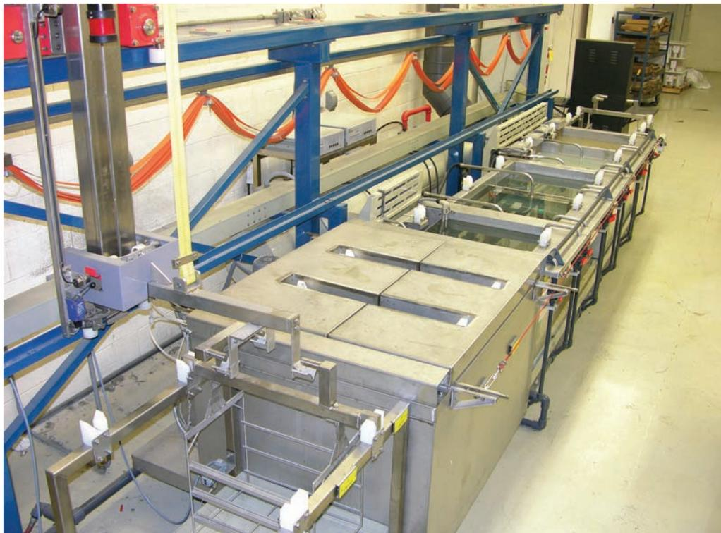
The anodize line has 27 stations, two fixed load and unload stations and 26 tanks.
