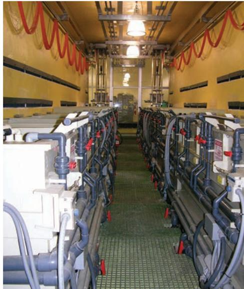
The system's two 1,500-lb. capacity programmed hoists are equipped with variable speed transfer motors.
